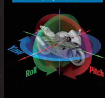
IMU/6-directions, along 3-axis, Pitch, Roll and Yaw
