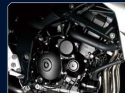
4-stroke, 4-cylinder, liquid-cooled, DOHC engine
