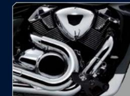
1,783cc<sup>1</sup> 4-stroke DOHC V-twin engine
