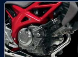
Fuel-injected, DOHC 90-degree V-Twin engine
