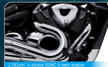
1,783cm<sup>3</sup> 4-stroke DOHC V-twin engine
