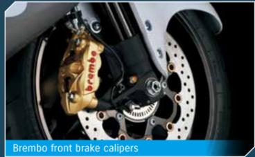
Brembo front brake calipers
