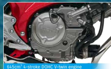
645cm<sup>3</sup> 4-stroke DOHC V-twin engine
