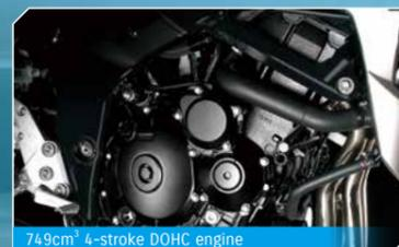
749cm<sup>3</sup> 4-stroke DOHC engine
