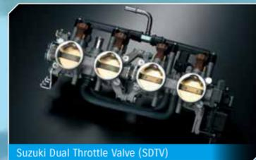
Suzuki Dual Throttle Valve (SDTV)
