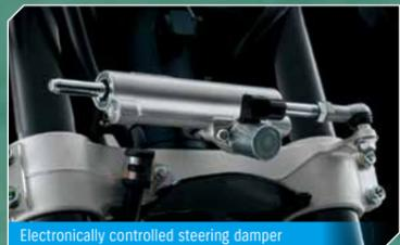
Electronically controlled steering damper
