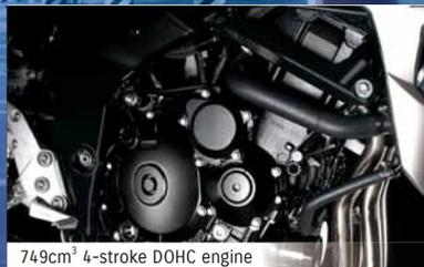
749cm<sup>3</sup> 4-stroke DOHC engine
