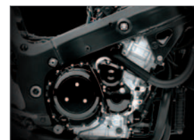
1340cm 3 4-stroke DOHC engine
