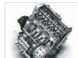
599cm 3 4-stroke DOHC engine
