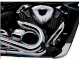
1,783cm 3 4-stroke DOHC V-twin engine
