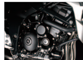
749cm³ 4-stroke DOHC engine
