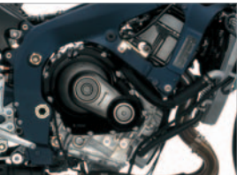
749cm 3 4-stroke DOHC engine
