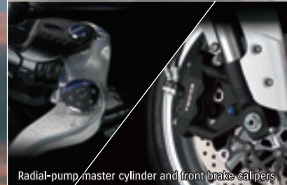
Radial-pump, master cylinder and front brake calipers
