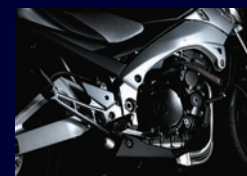
Aluminum frame and swingarm
