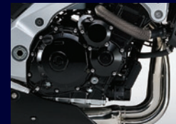
Liquid-cooled inline 4-cylinder, 4-stroke engine
